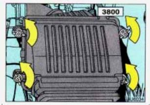
3800 V6: Checking Air Cleaner Filter Air Cleaner (CONT.)
