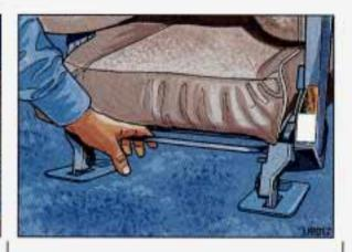
To get out of the third row seats, push down on the rear release bar under the seat ahead of you to tilt the seat forward.
