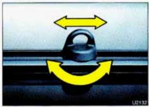
Use the adjustable tiedown loops in the side rails to help secure large loads. Reposition the tiedowns by turning them counterclockwise, then slide them along the side rail. Turn the tiedowns clockwise to tighten them in place.
