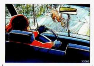
You can steer around the obstacle while braking hard. As you brake, your computer keeps receiving updates on wheel speed and controls braking pressure accordingly.
