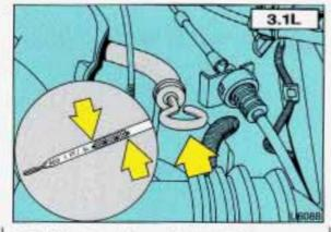
3.1L V6: Checking Automatic Transaxle Fluid
