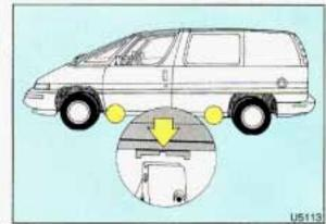
Loosen the wheel nuts—but do not remove them—using the folding wrench. Attach the folding wrench to the jack, and rotate the wrench clockwise to raise the jack head a few inches. 10. Near each wheel, there is a notch in the vehicle's frame. Position the jack and raise the jack head until it fits firmly into the notch in the vehicle's frame nearest the flat tire. Do not raise the vehicle yet. Put the compact spare tire near you.
