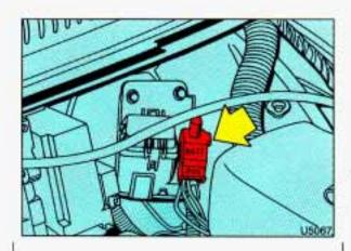
Your Oldsmobile has a remote positive (+) jump starting terminal. The terminal is in the red box on the same side of the engine compartment as your battery. You should always use the remote positive (+) terminal instead of the positive (+) terminal on your battery. To open the remote positive (+)
