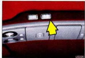
The sliding door must be unlocked for the power sliding door to operate. The key does not have to be in the ignition. To help avoid accidental operation of the sliding door, disable the power sliding door by placing the power sliding door override switch in the **OFF** position.
