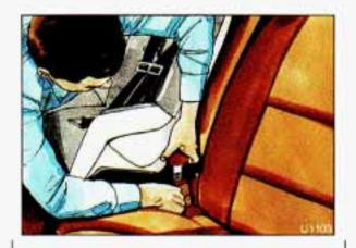
Buckle the belt. Make sure the release button faces upward or outward, so you'll be able to unbuckle it quickly if you ever need to.
