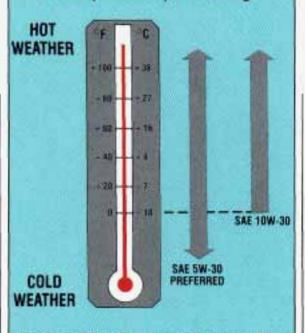
IF NEITHER SAE 5W-30 NOR SAE 10W-30 GRADE OILS ARE AVAILABLE, SAE 30 GRADE MAY BE USED AT TEMPERATURES ABOVE 40 DEGREES F (4 DEGREES C).
