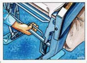
Then, from behind the seat, support the top portion of the seat with one hand as you squeeze the front release bar toward the crossbar. The seat will release from the floor pins.
