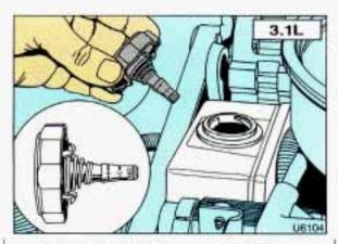
3.1L V6: Checking Power Steering Fluid
