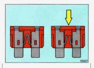
Look at the silver-colored band inside the fuse. If the band is broken or melted, replace the fuse. Be sure you replace a bad fuse with a new one of the correct size.
