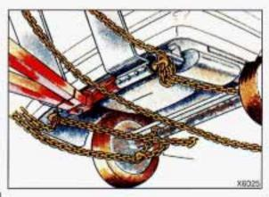
Position the lower sling crossbar directly under the rear bumper. No 4x4 wood beam is needed.
