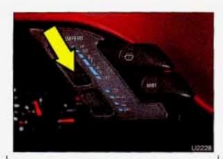
To Turn the Wipers Off: Slide the upper control to the OFF position.
