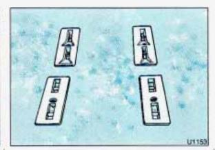
Push down on the rear release bar. The entire seat will tilt forward. 3. Then, from behind the seat, support the top portion of the seat with one hand as you squeeze the front release bar toward the crossbar. The seat will release from the floor pins.
