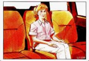
4. Position and release it the same way as the lap part of a lap-shoulder belt. If the belt isn't long enough, see the Index under Safety Belt Extender. Make sure the release button on the buckle faces upward or outward so you would be able to unbuckle it quickly if you ever had to.
