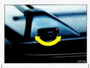
Your luggage carrier has release knobs set in the ends of each crossrail. Turn the release knobs counterclockwise, then slide the crossrails forward or back, as needed, to accommodate loads of varying size.
