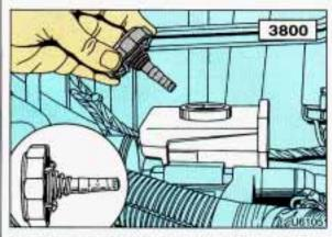
3800 V6: Checking Power Steering Fluid
