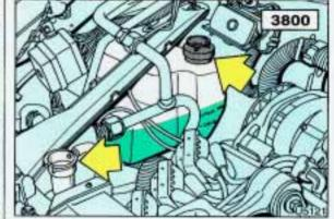
Fill the radiator with the proper mix, up to the base of the filler neck.
