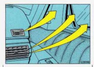
Your vehicle is equipped with side window defogger vents located on the top of the instrument panel. For additional side window defogging, press the **BI-LEV** button and adjust the fan to the highest speed. Aim the side vents on the instrument panel toward the side windows. For increased air flow to the side vents, close the center vents.
