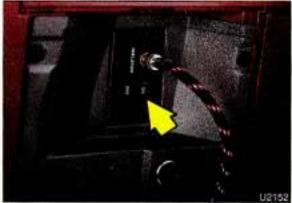
The air inflator kit is stored in a pouch in the glove box. It includes a 20-foot (6 m) hose with an air pressure gage, nozzle adapters and instructions.
